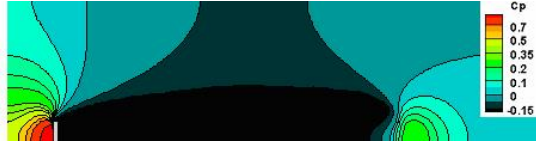
Fig. 15. Pressure coefficient for disk cavitator at \sigma = 0.15
