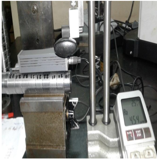
Fig. 5. Photograph of the surface roughness tester
