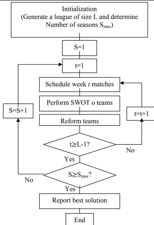
**Fig. 3. Flowchart for traditional LCA algorithm**
