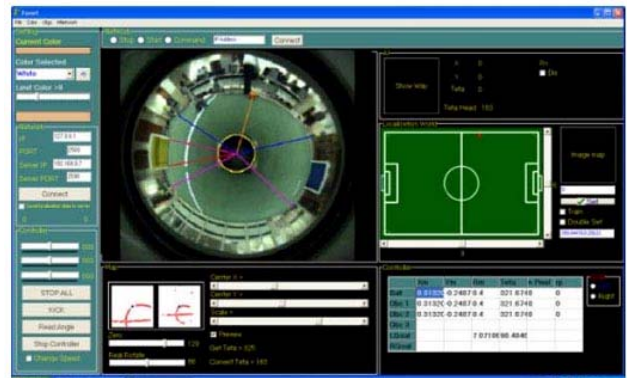
Fig. 7. Vision Systems, Object detection (Goals, Flag Spots, Ball)
