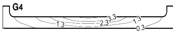
Fig. 8. Effective strain contour plot in G4 deformed at 1100°C and \omega = 10 rad.sec -1
