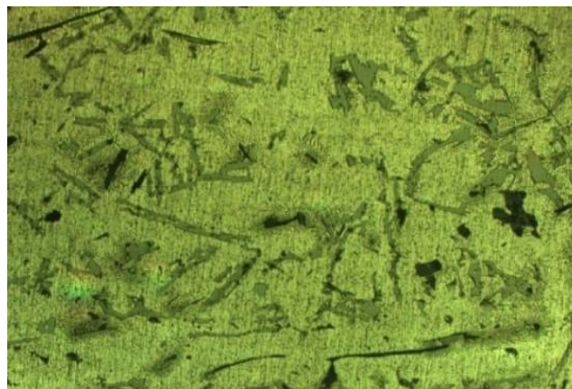
Fig. 5. Al 2124 microstructure after etching.
