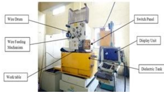
Fig. 2. Wire-Cut EDM set up photograph
