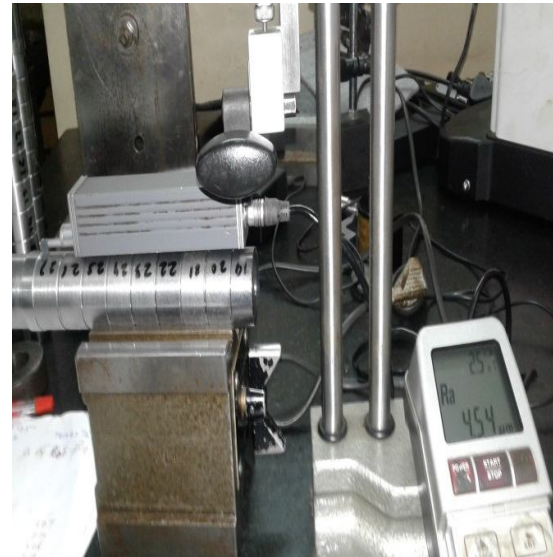
Fig. 5. Photograph of the surface roughness tester
