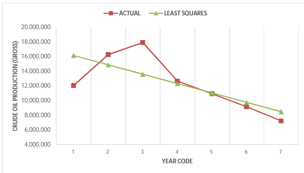
Fig. 3. The plot of the results of the least squares method of forecasting.
