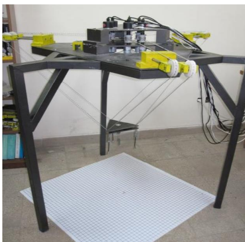
Fig.6. Space cable robot (ICaBot)
