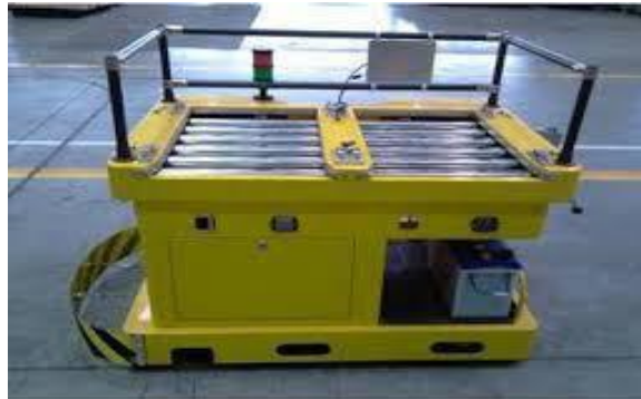
Fig. 2. A rail AGV
