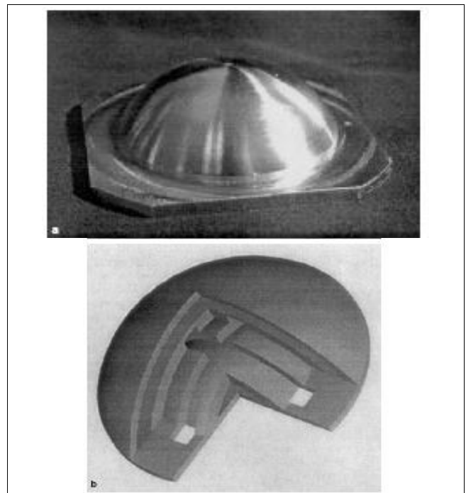
Fig. 3. (a) Manufactured part by microcasting (b) CAD representation of the part [1]
