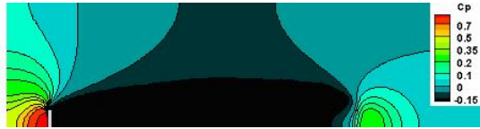
Fig. 15. Pressure coefficient for disk cavitator at \sigma = 0.15
