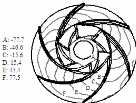
Fig. 8. The Static Pressure (KPa) Contours in Impeller when Handling the Oil ( \nu=62 \times 10^{-6} \text{ m}^2/\text{s} ).
