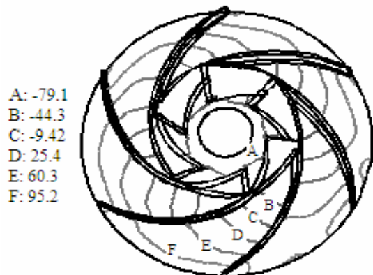
Fig. 6. The Static Pressure (KPa) Ccontours in Impeller when Handling the Water (v=1×10 -6 m 2 /s).
