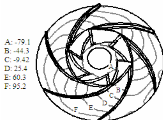
Fig. 6. The Static Pressure (KPa) Contours in Impeller when Handling the Water (v=1×10 -6 m 2 /s).
