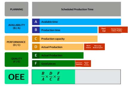
Fig. 4. Calculation method of OEE indicator.
