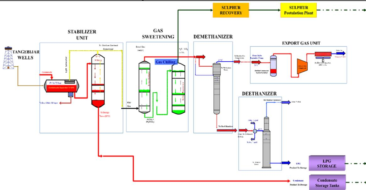
Fig.1. Structure of plant / refinery layout.
