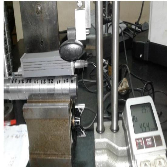
Fig. 5. Photograph of the surface roughness tester
