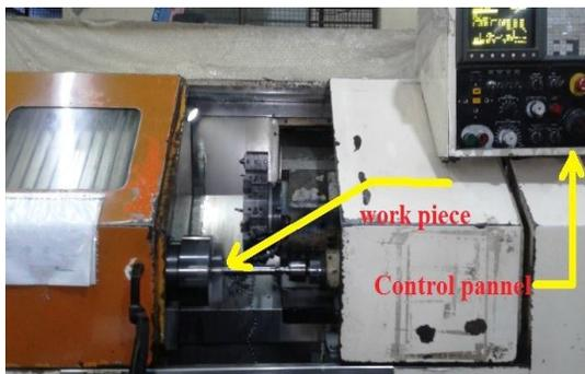
Fig. 2. CNC Lathe machine
