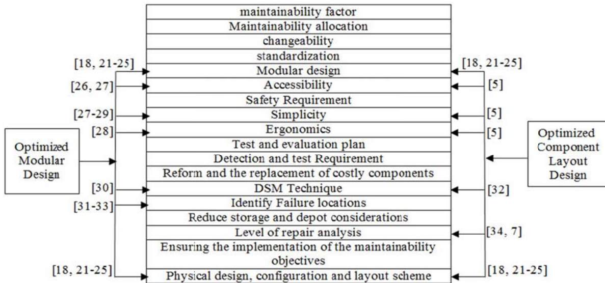
Figure1. Impact of layout and modular design on maintainability factors
