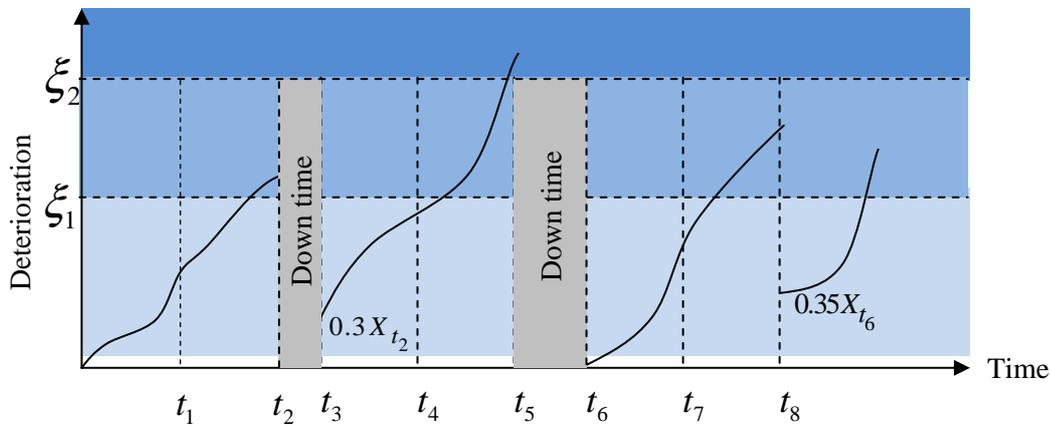
Fig. 1. Simulated behavior of the deteriorating system
