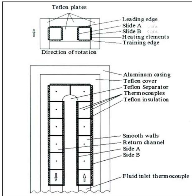
Fig 4. Heat transfer test model construction
