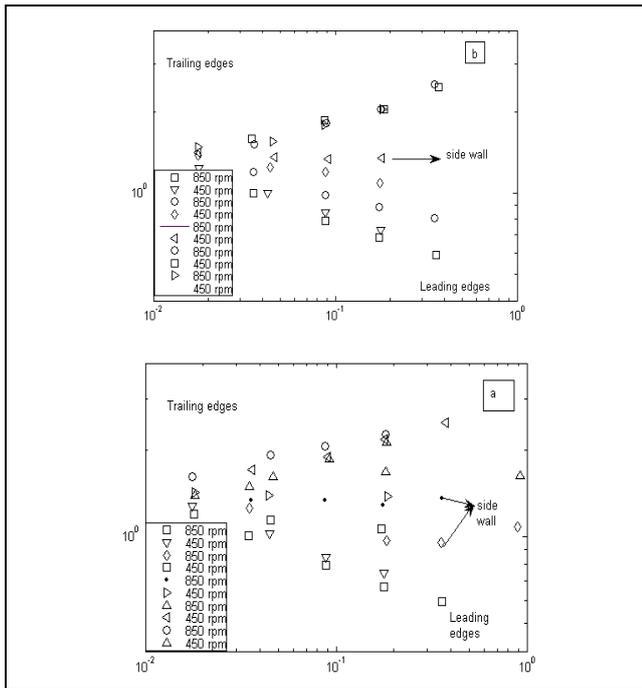
**Fig. 10 Influence of rotational number on average heat transfer ratio for situations (a) and (b), as well as (c)**
