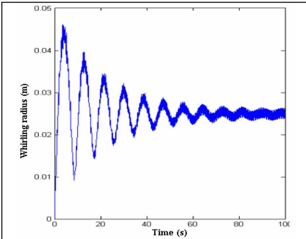
**Fig 4. Deflection at  $\Omega = 4.8$  rad/s for axial-lateral model**
