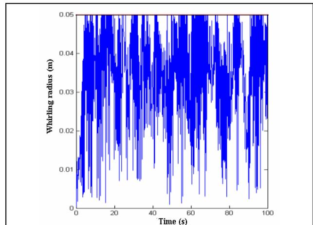
**Fig 7. Deflection at  $\Omega = 5.725$  rad/s for coupled model**
