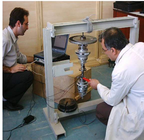
Fig. 6. Experiment setup for modal test of turbo-pump shaft in hammer test. Hammer, Accelerometer, and Data Acquisition unit are shown.
