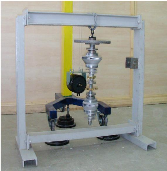
**Fig. 4. The Turbo-pump shaft, dangled from the support frame by a glued hook**
