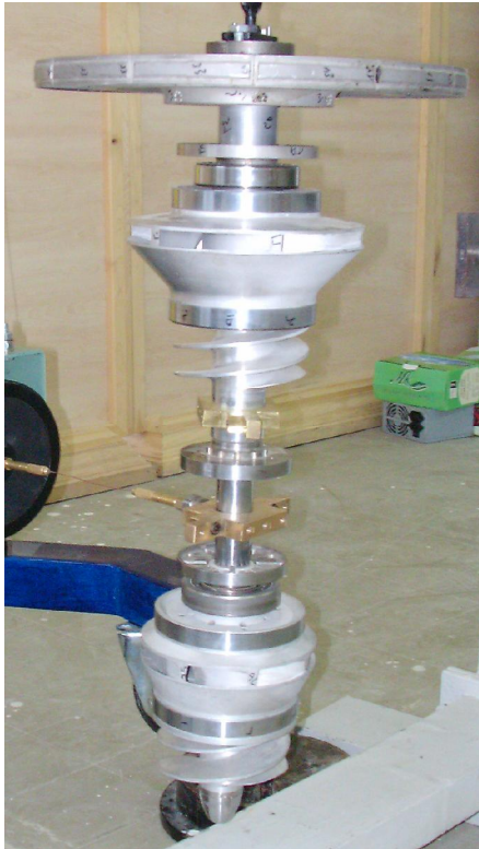
Fig. 1. The Shaft and corresponding components of turbo-pump
