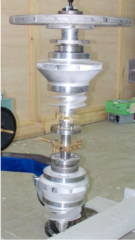
**Fig. 1. The Shaft and corresponding components of turbo-pump**
