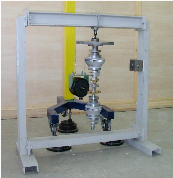
Fig. 4. The Turbo-pump shaft, dangled from the support frame by a glued hook
