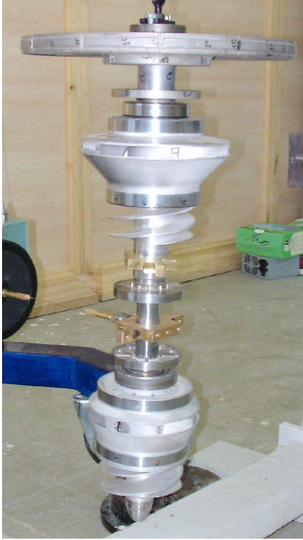
Fig. 1. The Shaft and corresponding components of turbo-pump
