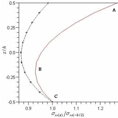
**Fig. 9. Non dimensional TRD of stresses vs. thickness in E-state with high rate temperature, dotted; timoshenko A-beam, cross; classical A-beam, solid; B-beam (Ni-Al<sub>2</sub>O<sub>3</sub>)**
