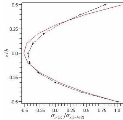
Fig. 8. Non dimensional TRD of stresses vs. thickness in E-state, dot line; Timoshenko's A-beam, cross; classical A-beam, solid line; B-beam (Ni-Al<sub>2</sub>O<sub>3</sub>)
