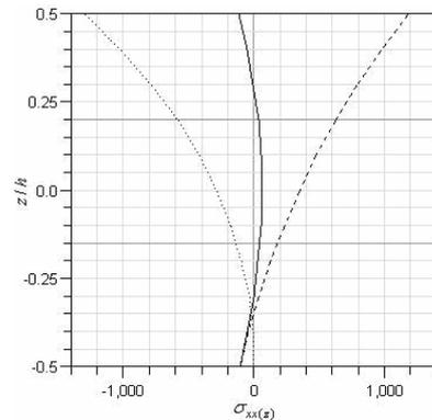
**Fig. 11. TRD of stresses (MPa) vs. thickness in H-state for B-beam, dotted; stress resultants of part A ( $\sigma^T$ ), dotted-dash; stress resultants of part B ( $\sigma^*$ ), solid; total stresses ( $\sigma$ )**
