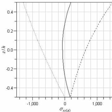
Fig. 14. TRD of stresses (MPa) vs. thickness in E-state for B-beam, dotted; stress resultants of part A ( $\sigma^T$ ), dotted-dash; stress resultants of part B ( $\sigma^*$ ), solid; total stresses ( $\sigma$ )
