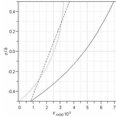
Fig. 15 TRD of strains vs. thickness in E-state for B-beam, dotted; strain resultants of part A ( $\epsilon^T$ ), dotted-dash; strain resultants of part B ( $\epsilon^*$ ), solid; total strains ( $\epsilon$ )
