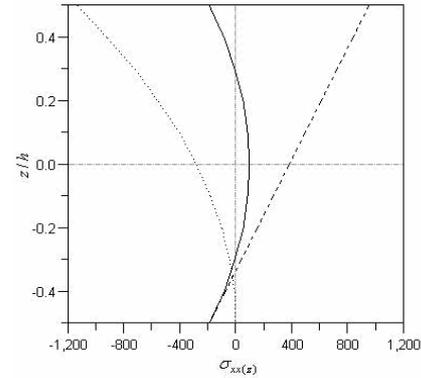
**Fig. 10. TRD of stresses (MPa) vs. thickness in H-state for classical A-beam, dotted; stress resultants of part A ( $\sigma^T$ ), dotted-dash; stress resultants of part B ( $\sigma^*$ ), solid; total stresses ( $\sigma$ )**
