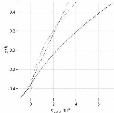
**Fig. 12. TRD of strains vs. thickness in H-state for classical A-beam, dotted; strain resultants of part A ( $\varepsilon^T$ ), dotted-dash; strain resultants of part B ( $\varepsilon^*$ ), solid; total strains ( $\varepsilon$ )**
