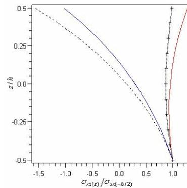
Fig. 16. Non dimensional stresses distribution vs. thickness for temperature boundary condition according to Eq.29 at the B-beam as exposed to thermo-mechanical load (E-state & External pressure on  $z/h = 0.5$ ), solid(right hand); thermal stresses, dotted(left hand); mechanical stresses, solid(left hand); total stresses
