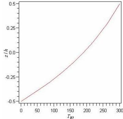
Fig.7. Exponentially distribution of heat in thickness direction of a beam
