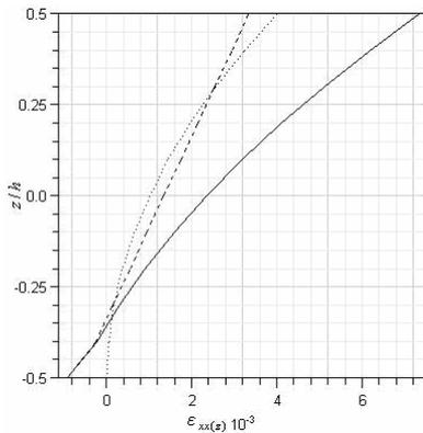
Fig. 13. TRD of strains vs. thickness in H-state for B-beam, dotted; strain resultants of part A ( $\epsilon^T$ ), dotted-dash; strain resultants of part B ( $\epsilon^*$ ), solid; total strains ( $\epsilon$ )
