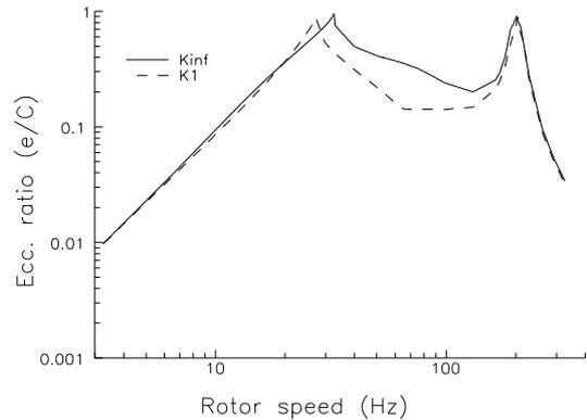
**Fig. 4. Predicted frequency response for the Jeffcott rotor, (dashed for supported damper, blank line for unsupported damper) (U=0.3, M2 = 0.25, ωr/ωc = 0.5, ωb/ωc = 0.3)**
