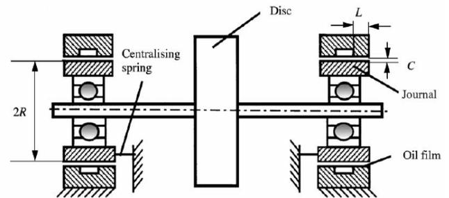
Fig. 1. Schematic of a flexible rotor bearing system
