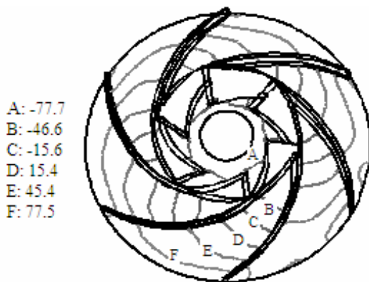
Fig. 8. The Static Pressure (KPa) Contours in Impeller when Handling the Oil ( \nu=62 \times 10^{-6} \text{ m}^2/\text{s} ).
