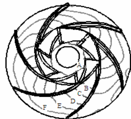
Fig. 6. The Static Pressure (KPa) Ccontours in Impeller when Handling the Water (v=1×10 -6 m 2 /s).
