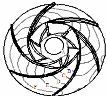
Fig. 6. The Static Pressure (KPa) Contours in Impeller when Handling the Water (ν=1×10 -6 m 2 /s).
