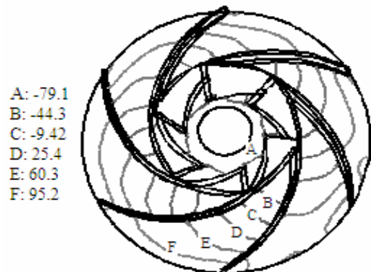
Fig. 6. The Static Pressure (KPa) Contours in Impeller when Handling the Water (ν=1×10 -6 m 2 /s).
