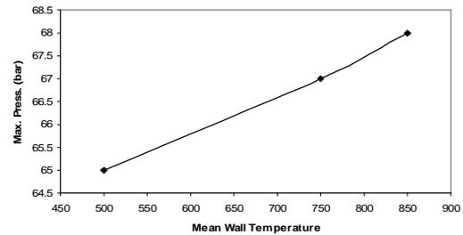
Fig. 13. Difference of Maximum Pressure Versus Mean Wall Temperature
