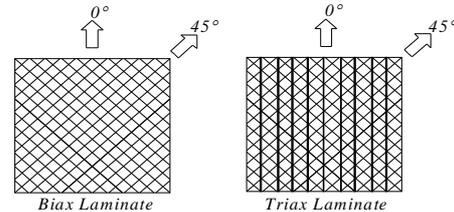
Fig. 3. Two Directions of Available Equivalent Elastic Modulus
